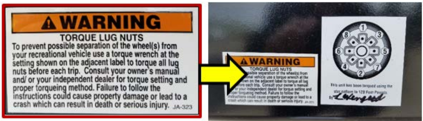
Lug nut torque pattern and warning label
